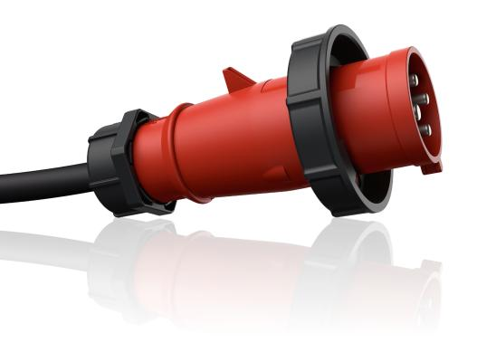
The new container plug with PE inverter fits 4-pin sockets with 3 h or 6 h clock position (32 A, 400-440 V) and supersedes the bad and illegal practise of removing the auxilliary nose.
