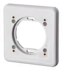
for panel mounted sockets of product groups 1733 and 1735. Using the flange, the sockets can be fitted on flush mounted installation boxes flange:  $106 \times 106 \text{ mm}$  / fixing hole spacing:  $60 \times 60 \text{ mm}$
